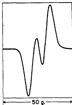
Figure 1. First derivative e.s.r. spectrum of the dianion radical III in dimethoxyethane.
